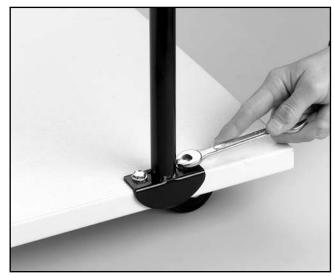
Figure 12. Mounting the brackets to the base.
